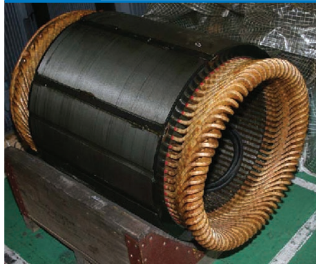
AC mill-duty stator before inserting in frame.
