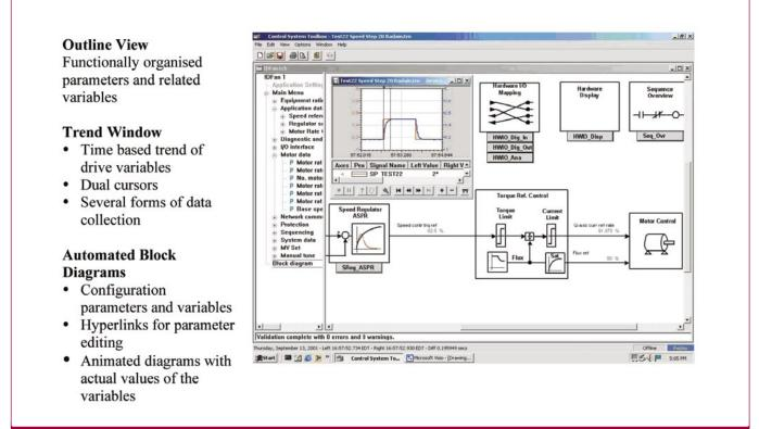
Drive Toolbox within LCMS for drive set-up and advanced diagnostics.
