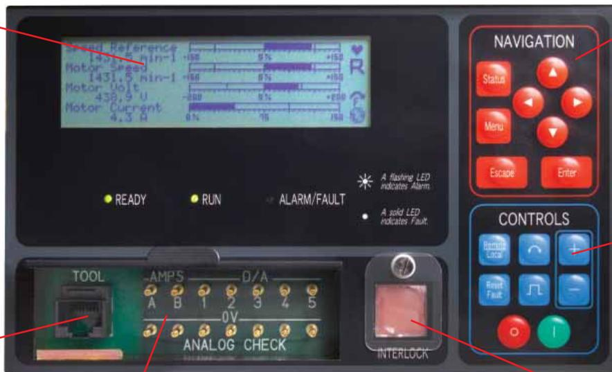
RJ-45 Ethernet port is used for the local Drive Navigator (toolbox) connection
