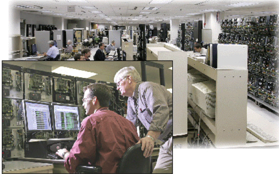
Test Lab showing Drive Simulators and HMI Screens
