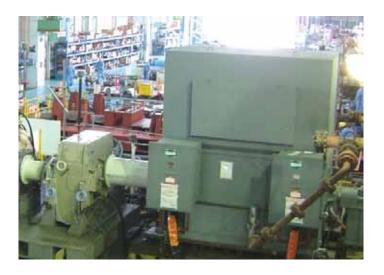
Expansion of the oil and gas industry has created demand for large motors to drive gas compressors and oil pumps. These motors are located in the production areas and on interstate pipelines, and are usually designed with explosion protection. For special applications such as driving large compressors and blowers, motor ratings can reach or exceed 100,000 hp.
