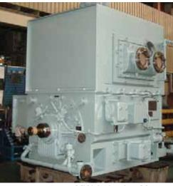
11,900 rpm, 1.8 MW, Induction Motor
