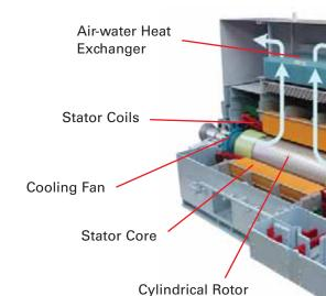
TMEIC builds a range of custom designed, highspeed, high-power synchronous motors for driving large compressors.
