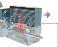
**Totally-Enclosed Air-Air** Cooled Type TEAAC/IP55 In a corrosive or harmful environment, a totally-enclosed fan-cooled motor can be applied. An external fan directs fresh air through the pipes in the air housing above the motor. The pipes serve as a heat exchanger in which outside fresh air passing through cools the hot air inside.
