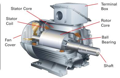
TM21-FII – Totally Enclosed Fan Cooled Internal Details
