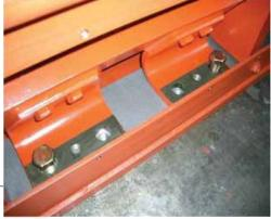
TMEIC unique spring-mounted stator design reduces vibration
