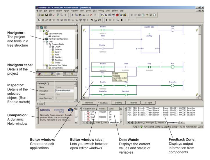
The screen above shows a typical layout of the tools and editors available. The editor window shows a ladder logic diagram with real-time data and power flow displayed in green. In addition to the windows shown above, two other windows can be added: **Toolchest**: This contains preconfigured objects that can be dragged into Machine Edition projects.
