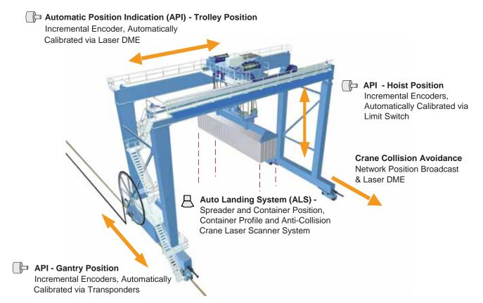
Automatic Position Indication System (API) – The API system makes direct measurements of the gantry, trolley, and hoist position via laser rangefinders, unaffected by factors such as rope stretch and wheel slippage.
