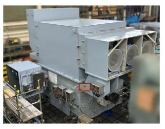
Air-air cooled 4-pole synchronous motor with low starting current at TMEIC's testing facility [Product range]
