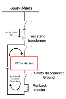
**Figure 3.** Runback reactor test set-up. © 2017 IEEE. Reprinted with permission.<sup>1</sup>
