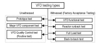
**Figure 2.** Types of large VFD testing types. © 2017 IEEE. Reprinted with permission.<sup>1</sup>
