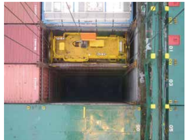
Spreader in cell (view from cabin)
