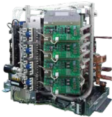
Water-cooled IEGT stack
