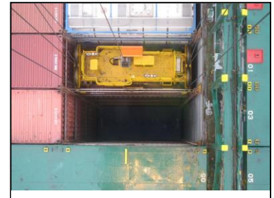
Figure 1 - Spreader in cell (view from cabin)
