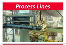
TMEIC has developed strip transport controls based on power analysis of all the elements, allowing high line speeds while eliminating problems such as strip breaks and bridle slippage. These advanced controls have demonstrated benefits including reduced operator intervention, maximized line throughput and uptime, and seamless product transitions.
