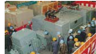
High-Speed, Two-pole, Synchronous Motor - 5,200 rpm
