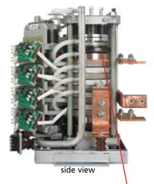
IEGT devices with integral forward and clamp diodes allow a very compact phase leg stack, reducing the footprint versus previous technology.
