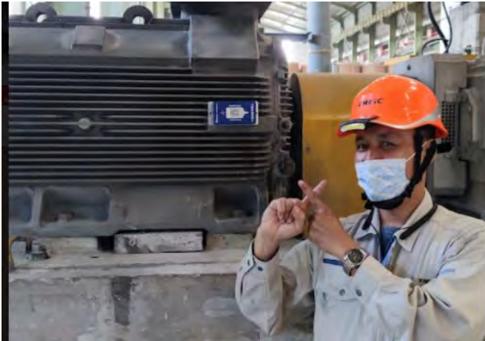
Device is not placed in the back area (in regards with the shaft of the motor)
