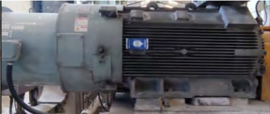
Correct installation of the SMS. Note that depending on the size of the motor, the SMS will take up more surface than what is shown in the sketch on the SMS case.
