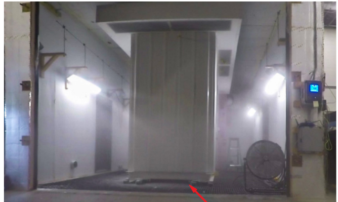
IMAGE 5: Outdoor MV VFD in environmental chamber (chamber door opened to show VFD inside)
