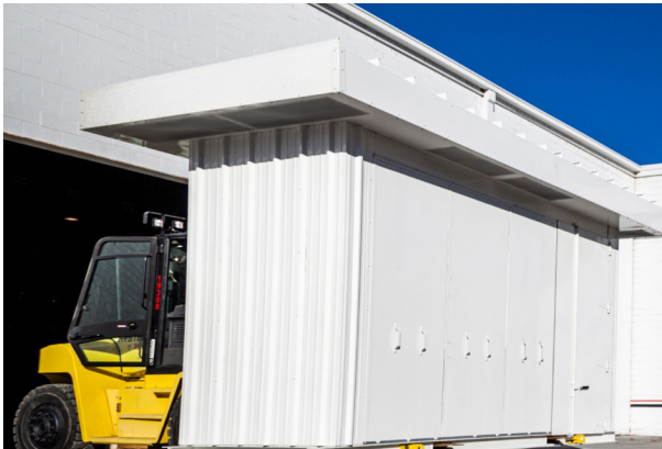
IMAGE 4: Outdoor MV VFD forklift test
