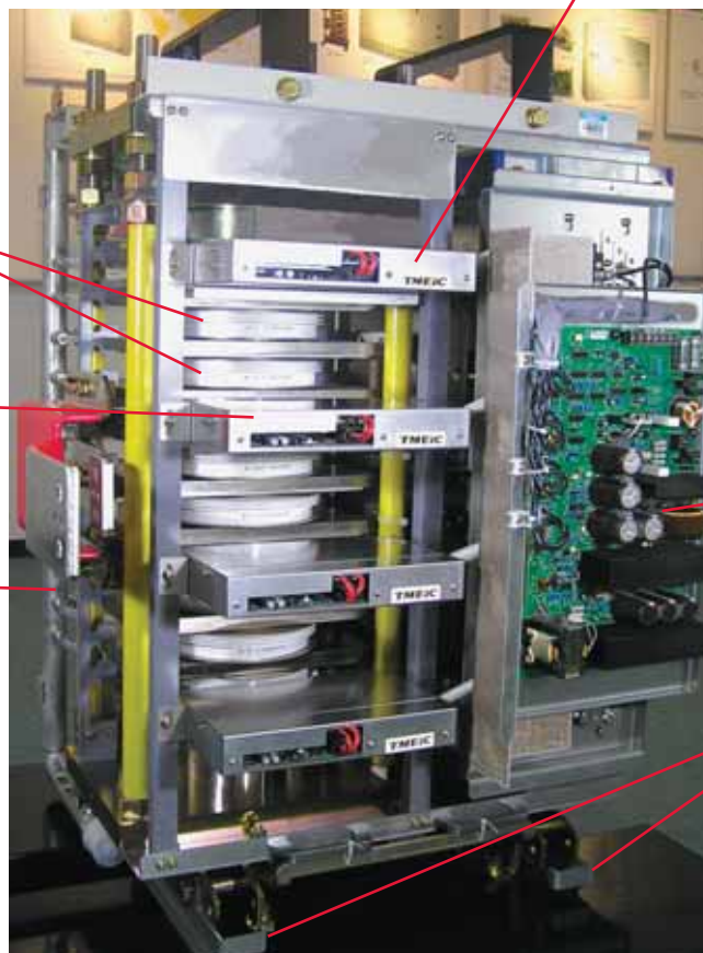
GCT Assembly showing firing circuits and control board, four per half-module
