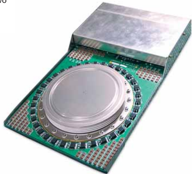
GCT Assembly showing firing circuits and control board, four per half-module
