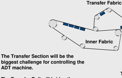
The Transfer Roll will bridge the \* Inner Fabric to the Dryer Fabric. Optionally, operator draw adjustment will be available for
