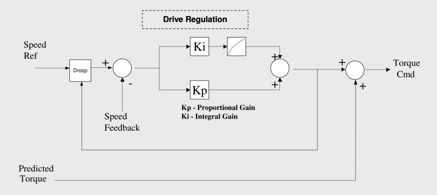
The above droop regulator is excellent for an application where low nip pressure "Soft Nip" exists between felts.
