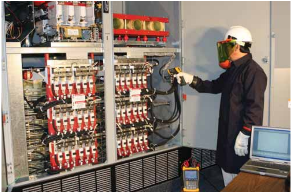
Dura-Bilt 5i MV Drive Factory Test
