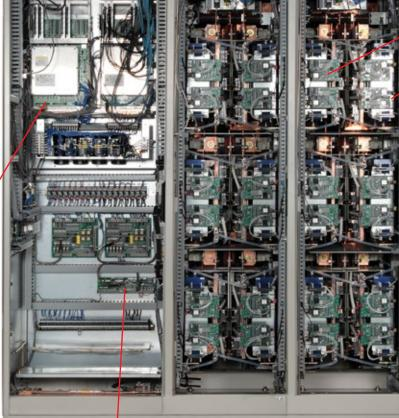
3 MVA Converter 3 MVA Inverter
