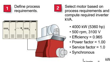
$kW_{Shaft} = 4000 \ kW \ (5360 \ hp)$ 500 rpm
