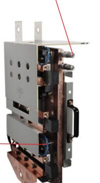
Dual IGBT Assembly common to inverter and converter section.
