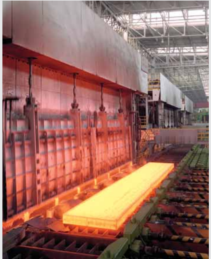
Steel Slab Exiting Furnace
