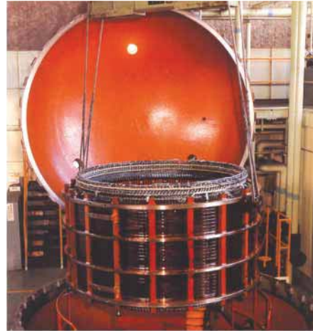
Vacuum pressurized impregnation process
