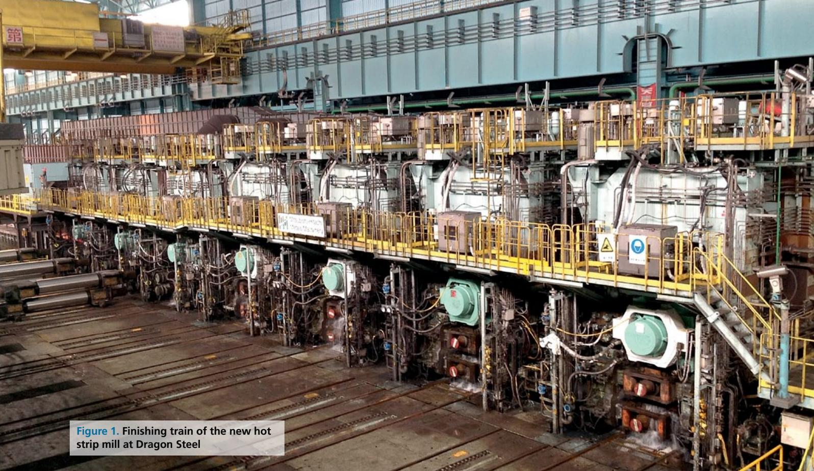
Figure 1. Finishing train of the new hot strip mill at Dragon Steel
