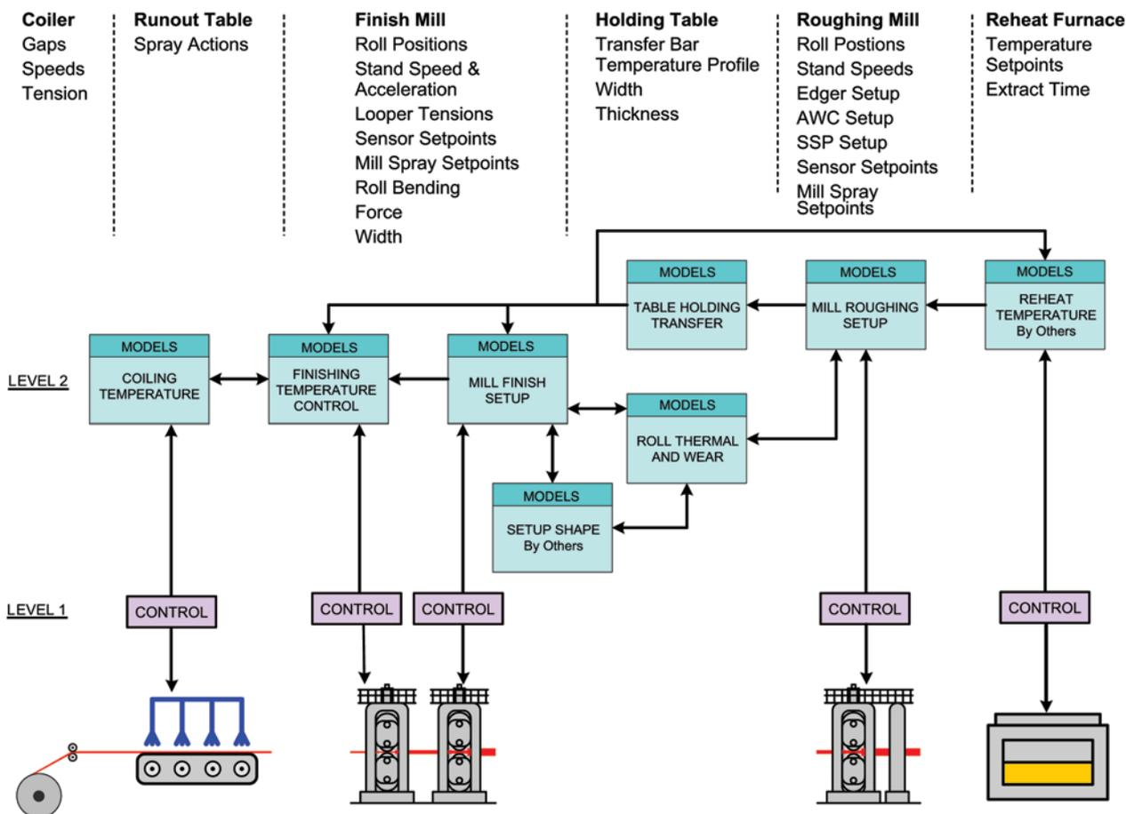
Figure 4. Level 2 models provide setup and references for the Level 1 control
