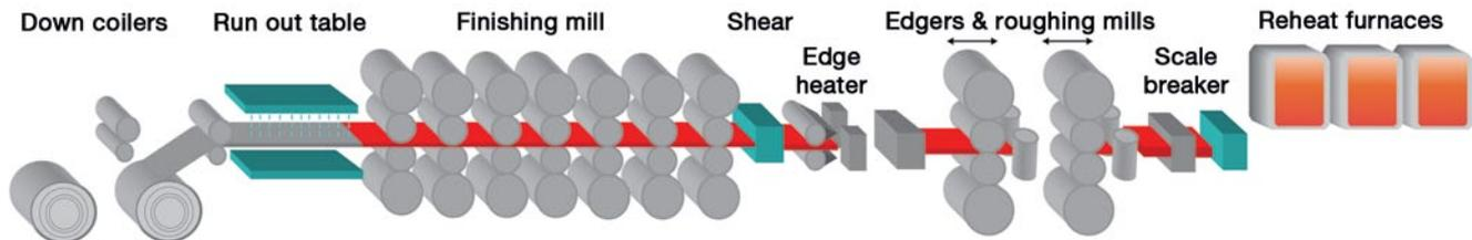
Figure 2. Diagram of the mill, metal slabs enter at right, coils are delivered at left
