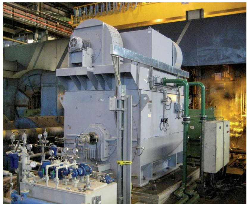
Figure 3. New induction motor and gearbox driving the cold mill
