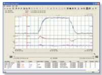
TMdrive-Navigator tool for configuration, monitoring & trending
