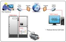
TMEIC engineers can quickly connect to the drive and diagnose many issues in minutes.
