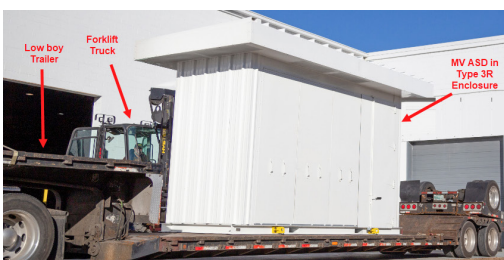
Image 5. Transport method and standard performance specifications of containerized outdoor MV drive
