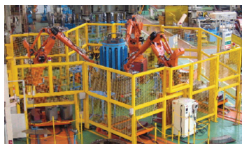
Robotic Stator Core Lamination Stacking
