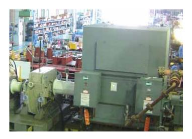
Expansion of the oil and gas industry has created demand for large motors to drive gas compressors and oil pumps. These motors are located in the production areas and on interstate pipelines, and are usually designed with explosion protection. For special applications such as driving large compressors and blowers, motor ratings can reach or exceed 100,000 hp.
