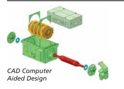
TMEIC motor engineers make extensive use of computer aided design to produce their detail and assembly drawings, both two-dimensional and three-dimensional.
