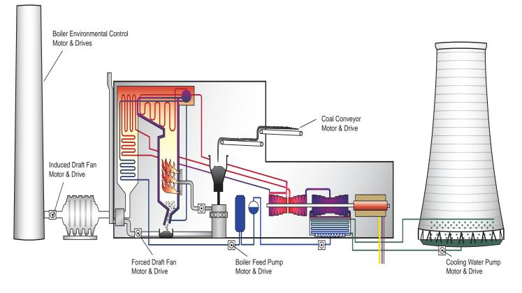
Controlling fan flow by adjusting speed avoids wasting energy in flow control vanes, dampers, and louvers. When large flows must be controlled and motor energy consumption is significant, varying the motor speed is the answer. With large machines, the electrical power savings can amount to hundreds of thousands of dollars per year. In addition, the drives smoothly start the motors, protecting them against starting inrush currents, thus avoiding thermal stress and extending motor life.
