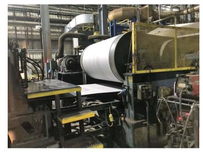
Figure 16, Entry Bridle was the first Dual Purpose drive
