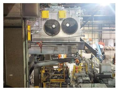
Figure 12, New Hot Bridle installed
