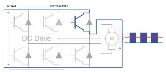
Figure 4, Inverter Bridge provides excitation for DC Motor Field<sup>1</sup>
