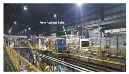
Figure 13, New Radiant Tube inserted between two existing Furnace Sections
