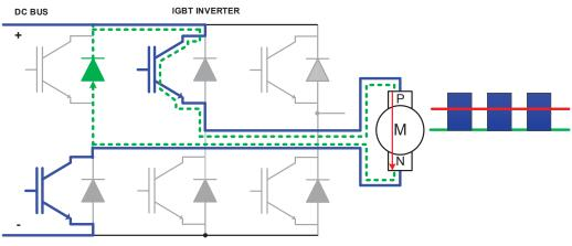
Figure 2, DC Motor Armature Positive Voltage case (Quadrant 1)<sup>1</sup>
