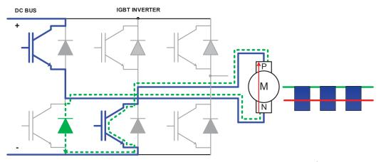
Figure 3, DC Motor Armature Negative Voltage case (Quadrant 3)<sup>1</sup>
