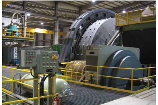
SAG Mill for grinding ore
