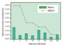
Typical Harmonic Contents of Input Current for 18-pulse System
