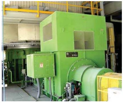
Synchronous Motor for Mill
