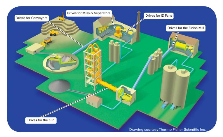
Controlling fan flow by adjusting speed avoids wasting energy in adjustable dampers and louvers. When large flows are involved and the motor energy consumption is significant, varying the speed is the answer. With large machines, the electrical power savings can amount to hundreds of thousands of dollars per year. In addition, the motors are protected against starting inrush currents, thus avoiding thermal stress and extending motor life.
