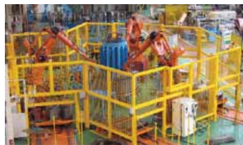
Robotic Stator Core Lamination Stacking
