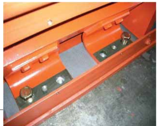
TMEIC unique spring-mounted stator design reduces vibration
