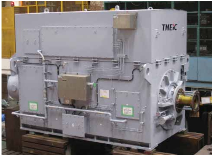
High Speed 25 MW 3,780 rpm Synchronous Motor
