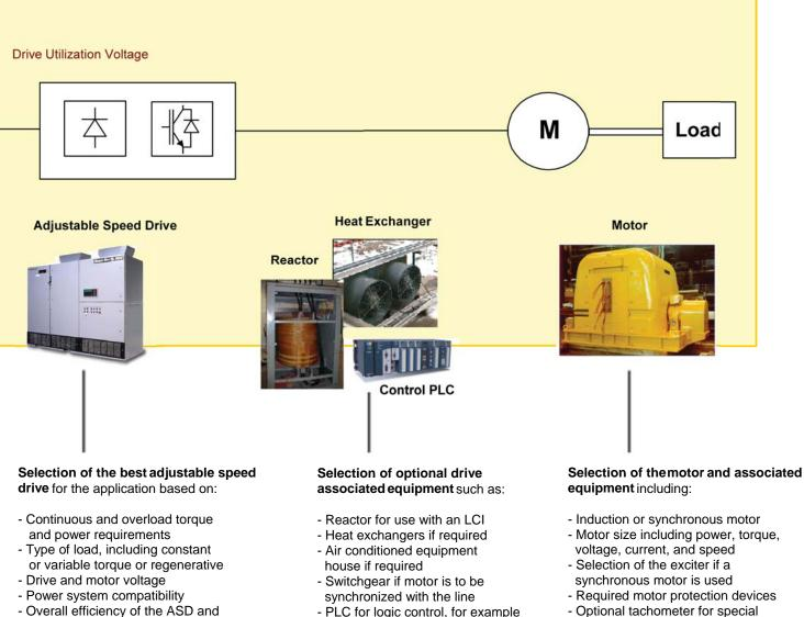
PLC for logic control, for example synchronizing multiple motors with the supply for soft start capability
