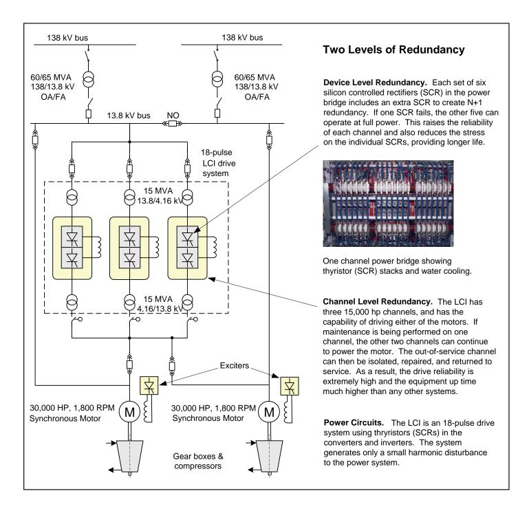
The two levels of redundancy illustrated above provide a 20-year system Mean Time Between Failures (MTBF) and excellent up-time with availability of 0.999994.
