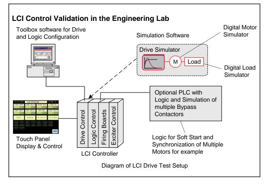
Validation of the optional LAN-DCS link and PLC sequencing and logic is done in the engineering lab using a simulated drive, motor, and load. Using the computersimulated equipment, the PLC is run through its sequencing and the resulting outputs validated.
