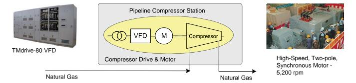
The TMdrive-80 high-speed GCT (Gate Commutated Turn-off Thyristor) inverter has the world's largest capacity. The GCT can operate at elevated speeds and be applied to voltages of 3.3 kV. The TMdrive-80 configuration perfectly fits large gas compressor applications.
