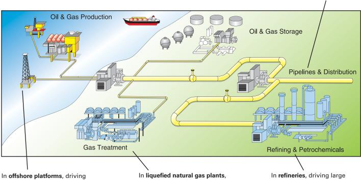
In **offshore platforms**, driving gas compressors and oil pumps, moving fluids to onshore – see Application 2, page 8. In **liquefied natural gas plants**, driving large compressors and varying speed to control flow – see Application 4, page 12. In **refineries**, driving large compressors and varying speed to control flow – see Application 1, page 6.
