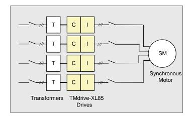
Simplified Block Diagram of Redundant VSD
