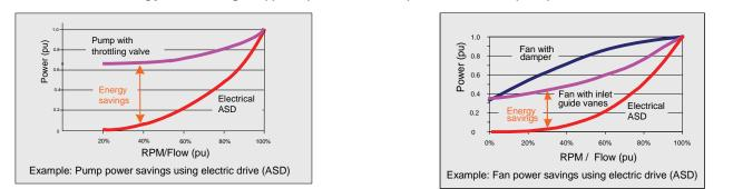
An example of the energy cost calculation for a pump driven by a motor and electric drive is shown below. The calculation for the mechanical system is similar and is described on the next page. Since energy consumption varies with speed and flow, you need the load profile table which shows the number of hours running at the various flows.
