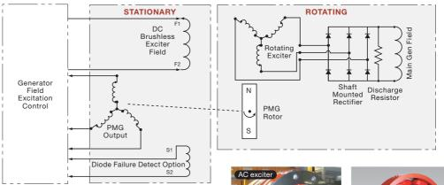
The brushless exciter and PMG wrap around the generator shaft, so additional bearings are not required. There is no collector ring nor carbon brush, so no carbon dust. As a result, daily inspections aren't required.
