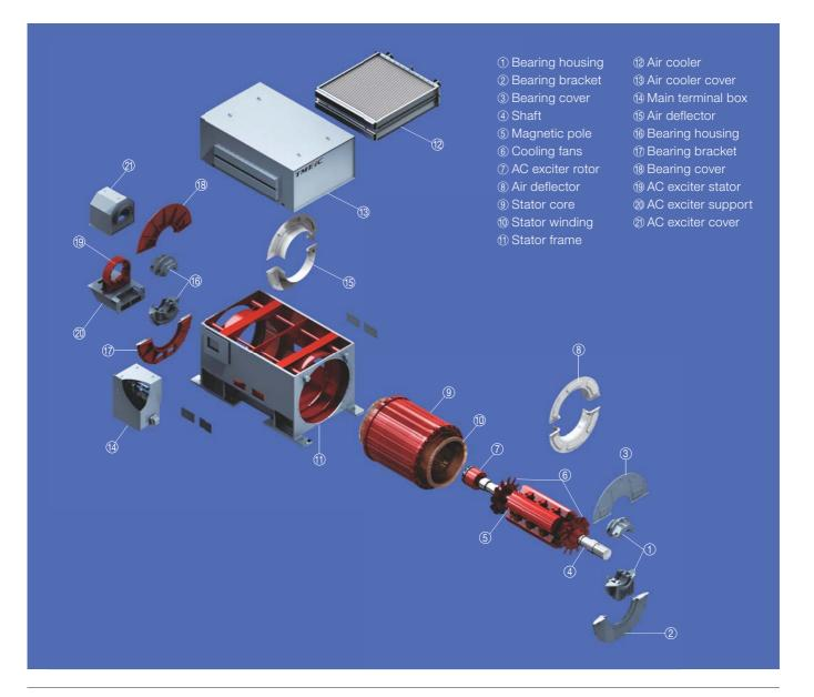
TMEIC 4-pole generators utilized in combination with steam or gas turbines equipped with reduction gears ensure highly reliable operation and optimum cost performance.
