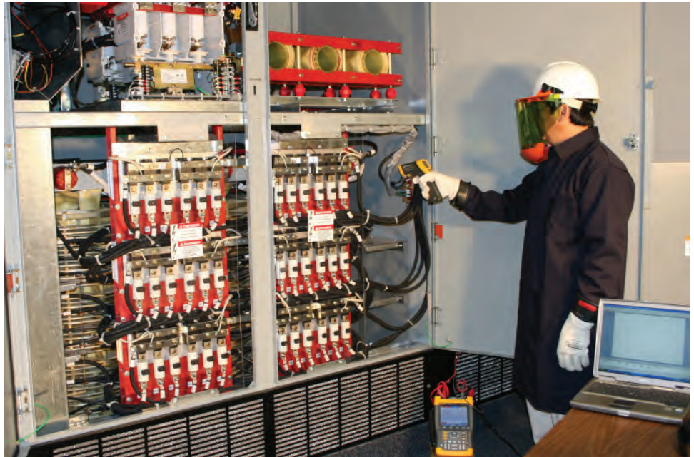
Dura-Bilt 5i MV Drive Factory Test
